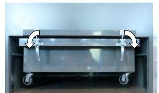
Before first start-up and after new filter cartridges are installed, a filter aid (pre-coating powder) must be introduced into the device. This forms a filter assist layer on the surface of the new filter cartridges and prevents dust particles from penetrating the filter cartridge. It increases the device's effectiveness, reduces caking, improves cleaning, and therefore lengthens filter cartridge life.
