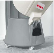
tilt the filter housing back up to vertical position. Remove the polyethylene collection bag and close it. Close the bag with the included cable ties so that it is dust-proof. Then close the opening again with the cap.
