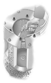
After the device shuts down, wait about a minute for the dust in the device to settle. Turn the cap counterclockwise to remove it from the filter housing.
