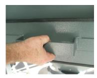
To do this, release the quick-tension locks on the drawer. Then the drawer can be removed and vacuumed out with an appropriate industrial dust extractor. After that, slide the drawer completely back into the raw gas collection container, and engage the quick-tension locks. The drawer must close firmly.
