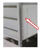
Loosen the inspection cover's fastening screws, and remove both cover and screws.
