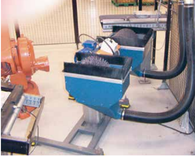
Robot deburring for telecom parts
