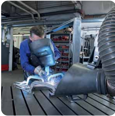
Extraction at the workplace
