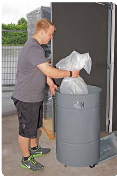
The mobile dust collection container with an inserted plastic bag allows easy, dust-free disposal of extracted dirt
