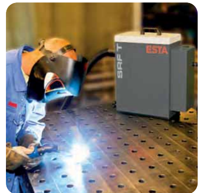
SRF T-2, direct extraction from one welding torch
