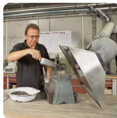
Square hood with baffle plate at a weighing station
