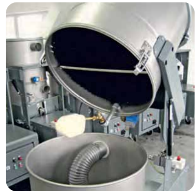
Tilt-back upper housing for easy access to the interior of the unit
