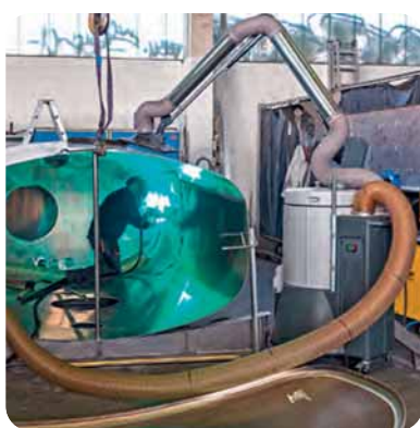
Extraction at the workplace
