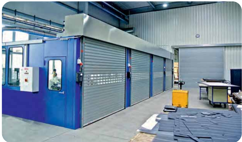
4-fold grinding cabin with rolling doors
