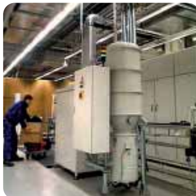
Cyclonic filter FZ-1003 with 100Litre collection container
