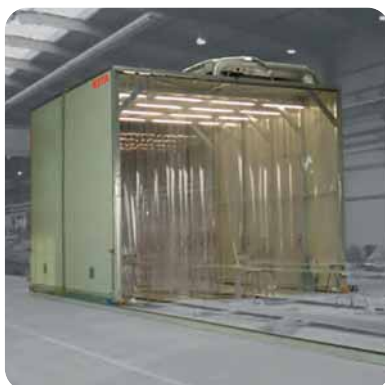
Mobile sanding station
